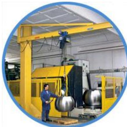
Standard over braced range of jib crane fitted with mains supply system & electric hoist ideal for machine shop applications were you need to use the hoist right next to the upright.
