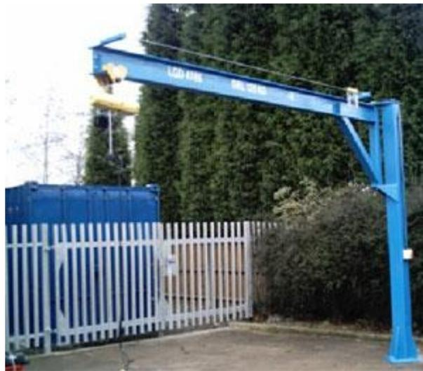
Our standard range which we make up to a safe working load of 3000Kg is a very cost effective lifting solution and is used in many industries whether to serve operating positions in machine shops or manufacturing plants or loading / off loading in stores etc.
