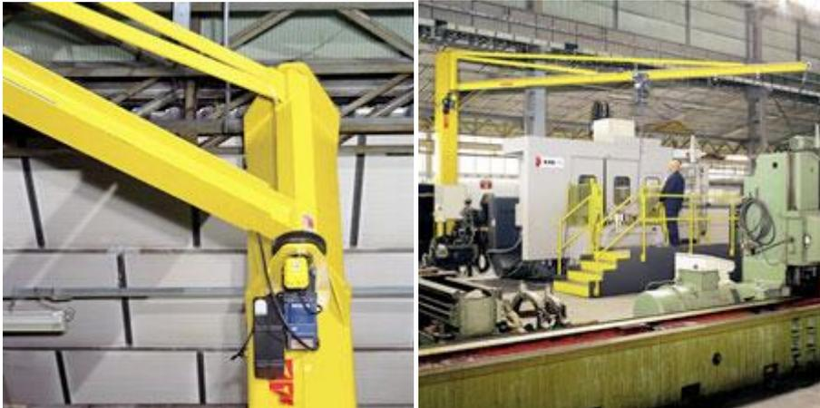
Our standard range of over braced swing jib crane can also be fitted with a motorised arm for higher and longer arm applications
